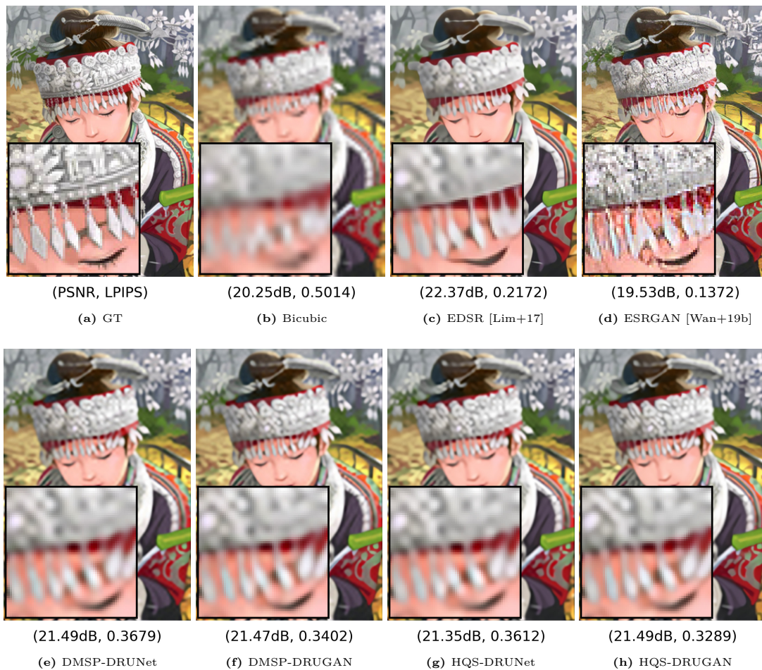
Figure 4.4: Single image super-resolution results on the image “Comic” of Set14 with bicubic downscaling
